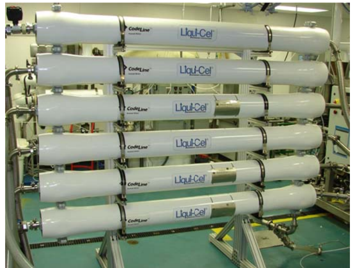
Liqui-Cel® 8 x 80-inch high pressure ASME code rated degassing system
