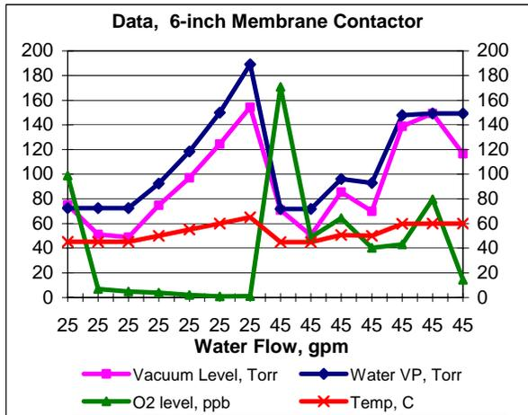
A review of the data shown in the graph indicates several very important points regarding the use of a membrane contactor for this application. An initial key point is that dissolved oxygen levels can be reduced to well below 10.0 ppb with a single contactor. In more “traditional” membrane contactor designs several contactors in series are typically required to reach these lower levels of dissolved oxygen.
