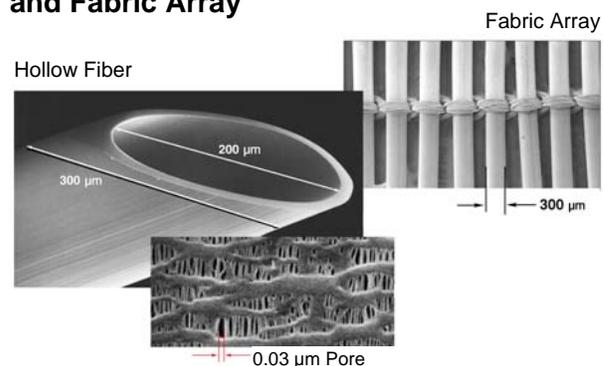
With the fiber array wrapped around the distribution tube, the fiber ends can be potted and then cut to length to complete a finished cartridge. This cartridge design creates a bundle of hollow fibers. These fibers are arranged parallel to the distribution tube.
