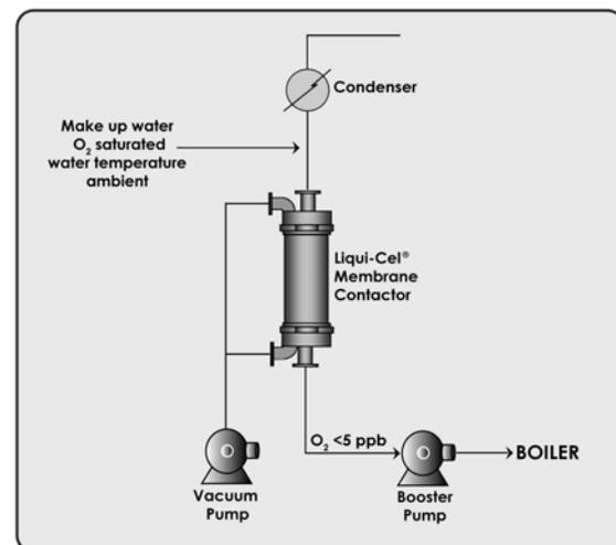
In Figure 5 the basic system in which this work was conducted is illustrated. In this work, tests were conducted over a range of flow rates,
